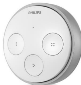
Figure 22: Hue Tap, each button activates a scene configured in the app. (smarthome.com.au)
