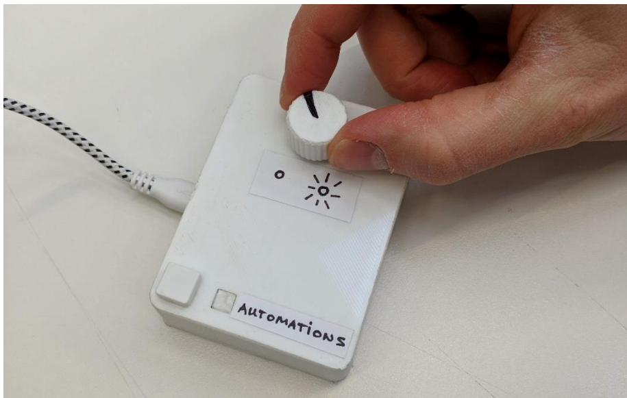
Figure 34: Scenario 2, the first dimmer prototype with a user changing the brightness
