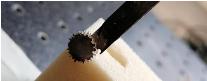
Figure 68: The first iteration of the prototype after failure during the straight trajectory drilling test.
