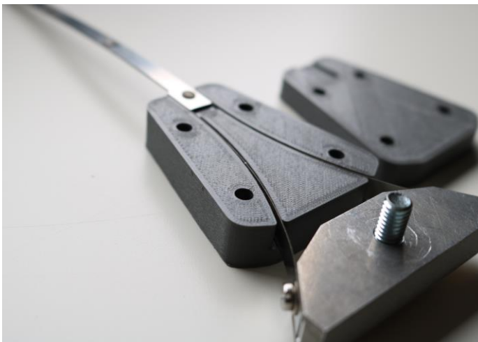
Figure 26: A closeup of the 3D printed guiding parts containing the flexible transmission.
