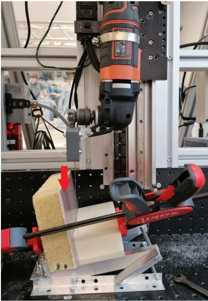
Figure 35: The experimental setup for curved trajectory drilling with the prototype. A block of foam is clamped onto the simulated cortical wall, which is indicated by the red arrow, and placed at an angle below the prototype.
