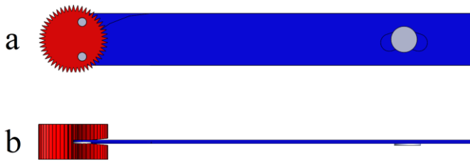
Figure 19: A model of the cutting head and the two leaf springs. a) A side view showing the two hinge pins in the cutting head, and the curved slot in the leaf springs. b) A top view showing the slot in which the leaf springs are mounted. Note that the slot widens at the outside of the cutting head, which ensures the teeth do not damage the springs when the device is bent.
