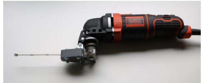
Figure 27: The complete prototype of the vertebral drilling device, including the oscillating actuator.
