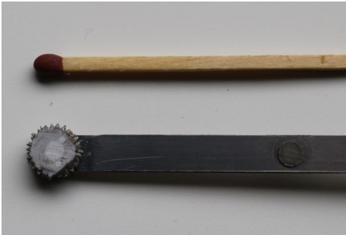
Figure 25: A closeup of the cutting head with a match stick as a reference. Note that the pins in the cutting head are visible.
