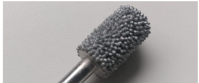
Figure 18: The Dremel 9933 tungsten carbide cutter that was used for the cutting head.
