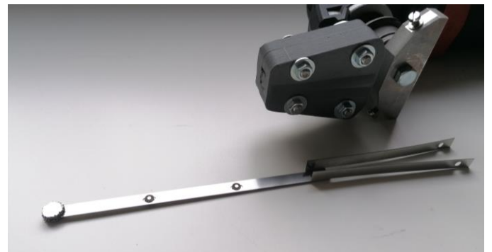
Figure 28: The second iteration of the prototype, with 0.3 mm thick leaf springs.
