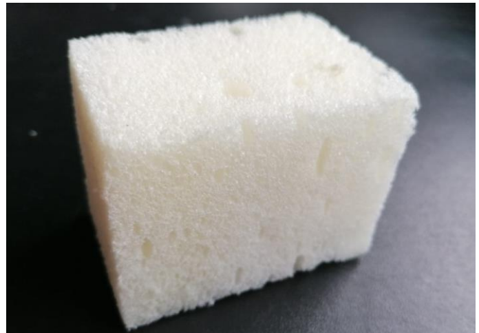
Figure 58: One of the blocks of polyurethane used as a cancellous bone phantom.
