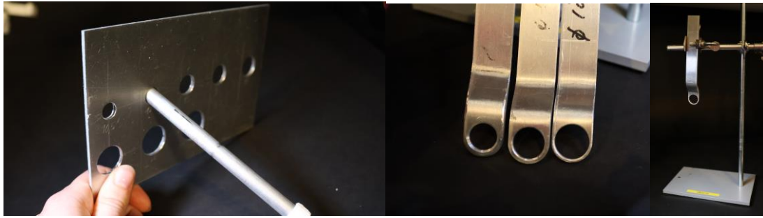
Figure 37 Metal plate with different hole sizes, the 3 produced holders in 14.5 16.5 and 18.5 mm and set up
