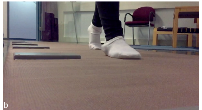
Figure 24. The GAITRite™ 7-meter Walkway in test setting including control monitors for video recording and control of the two measurement systems (a) and the insoles taped under the feet, stabilized with outer-sock (b).
