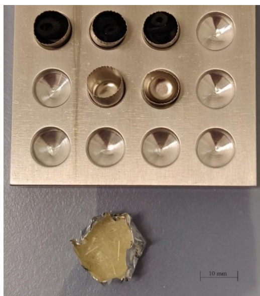
Fig.6-1. Samples in aluminium capsules ready to be tested in \mu -VCM facility.
