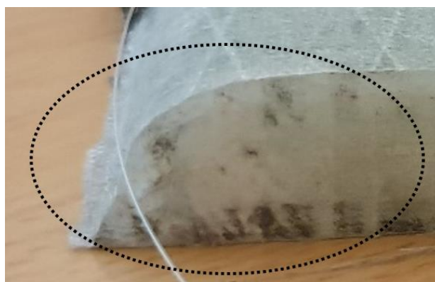
Fig.5-12. Rounded down edges of 1 mm thick composite after the manufacturing process.
