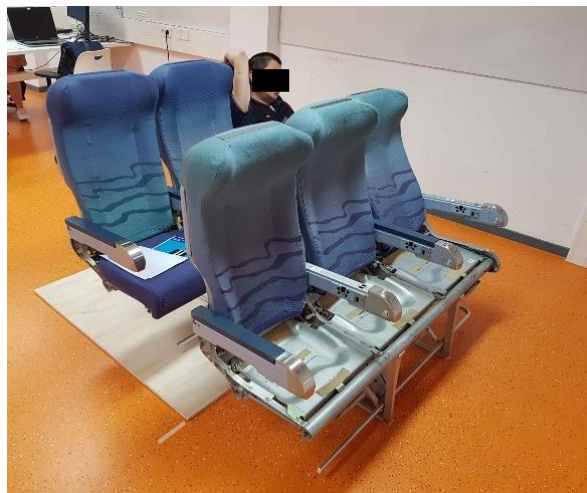
Figure 4.5 The traditional seats used in the test. Participants were asked to sit in the 2 nd row. The seat pitch was set as 32'' as well
