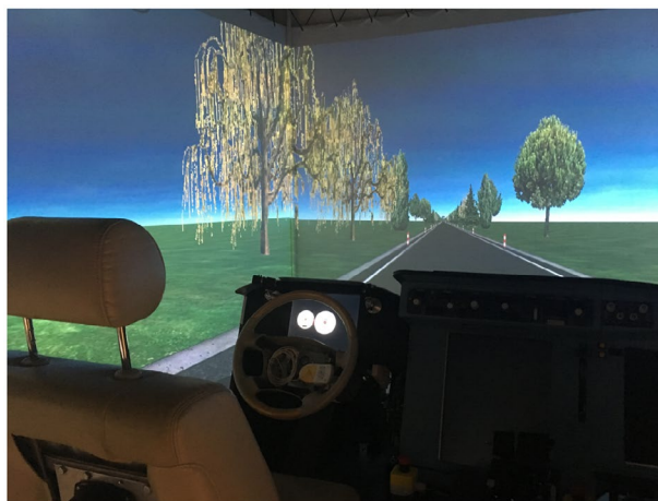
Figure 2. The fixed-based driving simulator used for the experiment.
