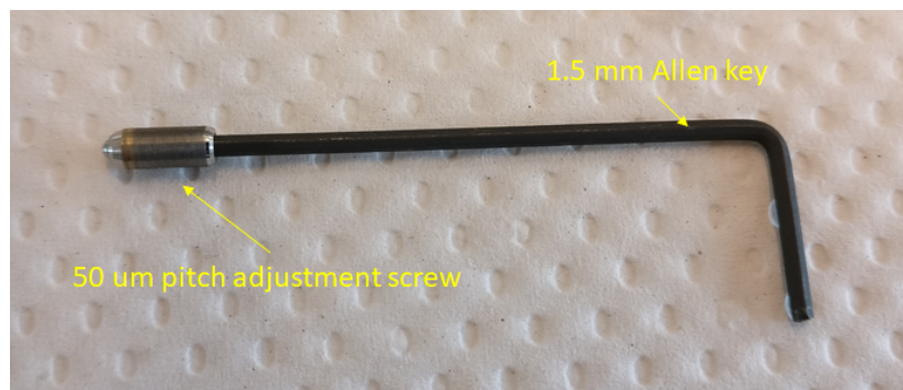
Figure 8.4: 50 \mu\text{m} pitch adjustment screw with a 1.5 mm Allen key.
