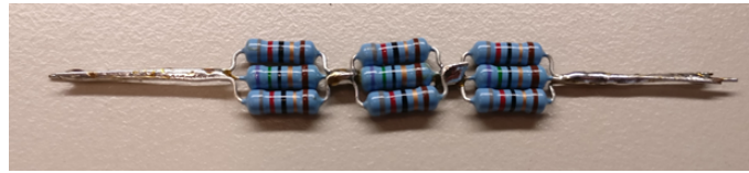
Figure 9.10: Set of resistors used for dissipating 0.6 W into three collimator dummies.
