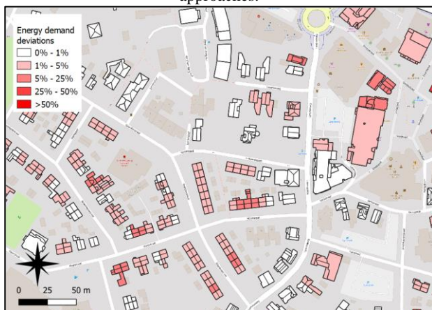
Figure 8. 2D visualisation of the energy demand deviations (in %) between hybrid and fully 3D approach.
