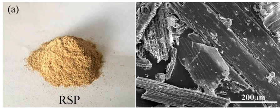
FIGURE 1 (A) particle morphology and (B) SEM morphology of rice straw powder.
