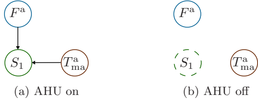
Figure 6: Bayesian network representations of case study 1. During day symptom S_1 is influenced by both an AHU fault and by the mixed air temperature. During night, the AHU is switched off and the relations between F^a , T_{ma}^a , and S_1 no longer hold.
