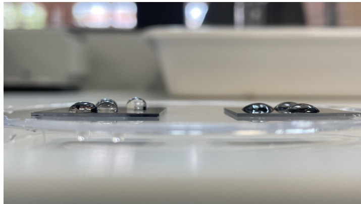
Figure B.8: Picture of the result of coating the molds with TCPFOS, showing the contact angle of demineralized water. On the left is the coated substrate, while on the right is an uncoated substrate.
