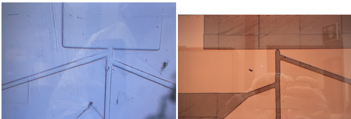
Figure B.2: The result of printing the first design with the Micro2 SLA (left) and the Nanoscribe 2PP (right) printers.
