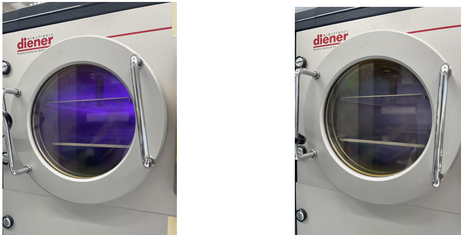
(a) Chamber during air plasma exposure (indicated by the purple glow). (b) Chamber during oxygen plasma exposure (indicated by the grey glow).
