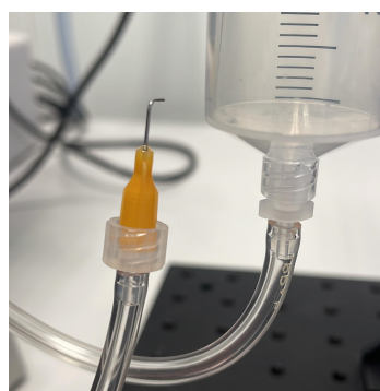
(c) Photo showing the connection parts: Luer lock connections (Darwin Microfluidics, SKU: MF-45518-02 & SKU: ID-P-858), tubing (Darwin Microfluidics, SKU: SA-ACF00005) and bend dispenser tips (Nordson EFD PN: 7018316).
