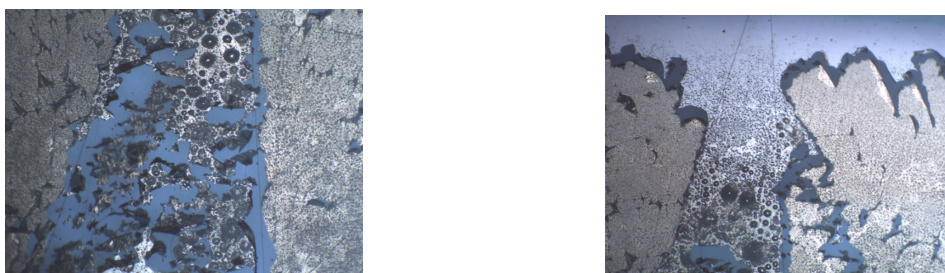
Figure B.15: Optical microscope images of the sputter coated gold electrode after flushing of the microfluidic system. It can be seen that in regions where fluid flows over the electrode, the gold is removed.
