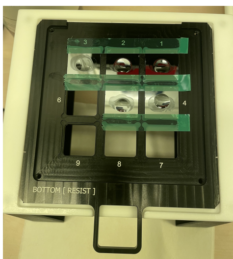
Figure B.6: A photo of the substrates with resin mounted to the sample holder.
