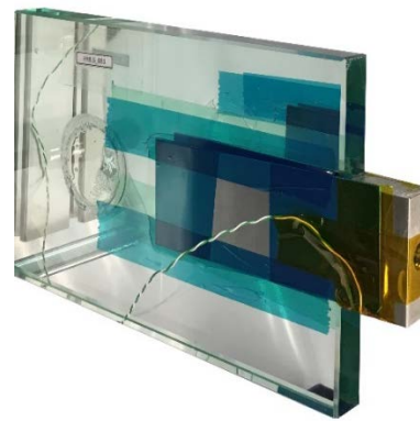
Fig. 2 Edge-laminated connection during fabrication process
