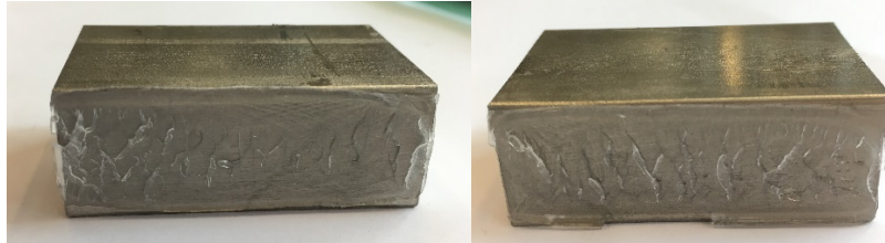
Fig. 9 TSSA laminated connections on the glass edge after failure
