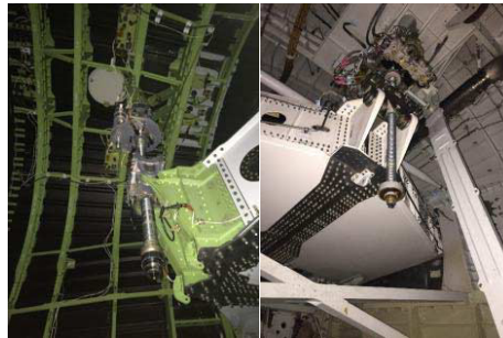
Figure 5. Elevator trim screw jack. Left 787-8. Right A320-200.
