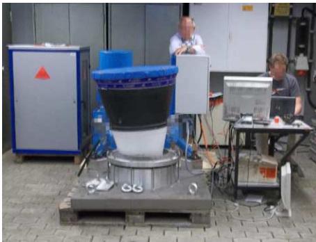
Figure 7. Engineering model of actuation system at transferor.
