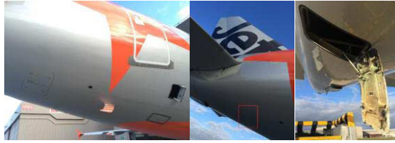
Figure 4. Location of access hatch on A320-200 aft of the rear pressure bulkhead.
