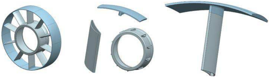
Figure 3. Welding assembly sequence of a structural jet engine component.
