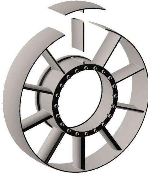
Figure 4. Static turbine part.
