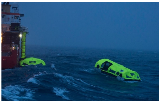
Figure 1.6: Flexible life raft deployed next to a ship in heavy sea conditions[98]
