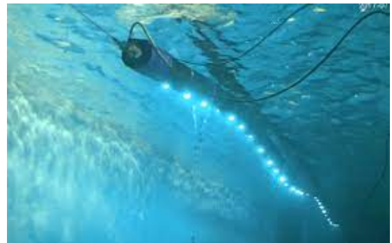
Figure 1.7: Flexible Wave Energy Converter Prototype by SBM Offshore, being tested in a pool [65]
