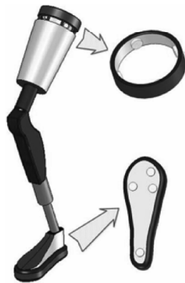
Figure 39: Conceptual model of the lower-limb prosthesis with a cuff placed around the thigh. In this cuff PBAs are placed. Sensors on the bottom of the foot translate pressure information into the inflation of the PBAs [36].
