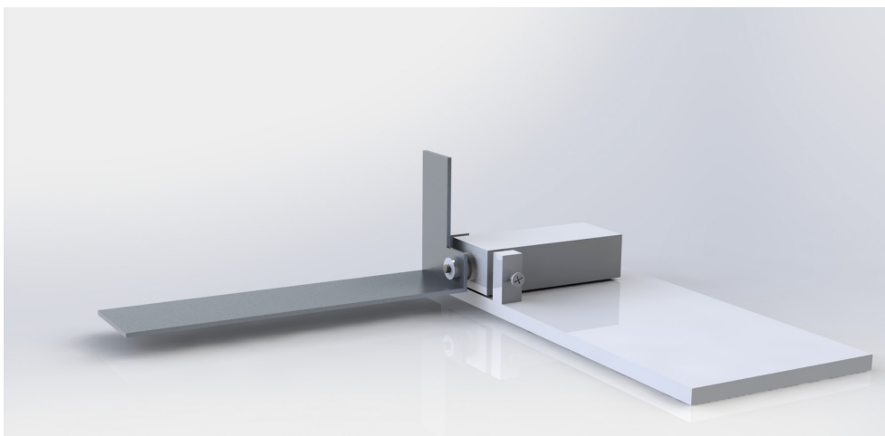
Figure 5.9: Base showing that the cylinder is fixed inside a block, but is able to rotate because of the hinge joint.
