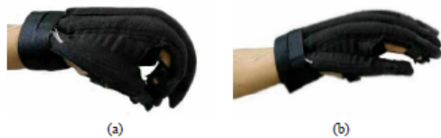
Figure 32: A pneumatic bending actuator with a spring inserted to create a bidirectional rehabilitation glove. (a) The actuator was not inflated, so the spring causes the bent position. (b) The actuator was inflated, which causes the extended position [86].
