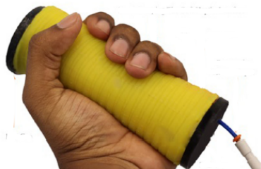
Figure 41: A soft robotic interface with force-control [76].
