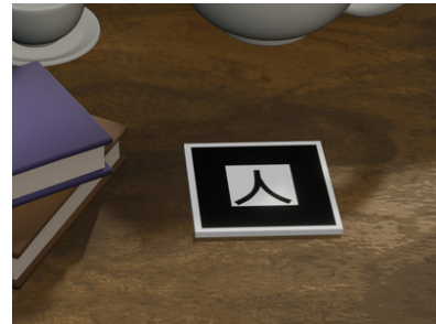
Figure 5: Example of a typical marker used in AR scenes. Identified by a unique shape surrounded by a thick black border.
