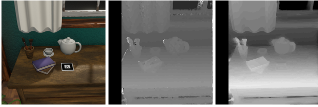
Figure 6: The steps involved in converting stereo images (left), to disparity maps (middle), to filtered disparity maps (right). Only the respective versions of the left stereo image is shown (with increased contrast).
