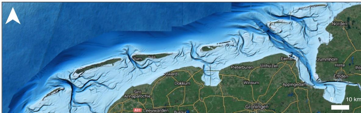
Figure 3.3: Visualisation of the bathymetry of the Dutch Wadden Sea from a *vaklodingen* data set. Deep areas such as the tidal channels are depicted in dark blue, whereas shallow waters such as the tidal flats are shown in light colours.
