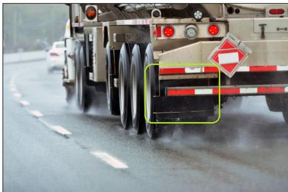
Figure 1.2: Mudflaps (in green box) attached to the underbody to minimize jetting of fluid behind wheels.
