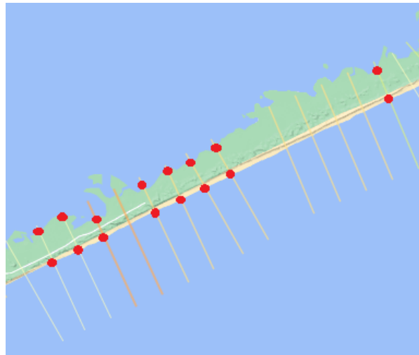
Figure 2.1: Example of a location (Fire Island, US) where the length of the transect exceeds the width of the coast. The red dots indicate the identification of a coastline at a transect with a length exceeding the width of the barrier island.
