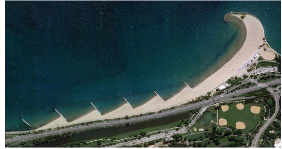
(d) Sand accumulation at a system of groynes at North Avenue Beach in Chicago, USA. (source: pruned.blogspot.com)
