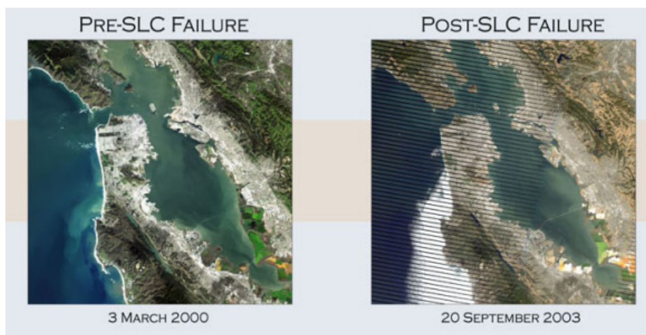
Figure B.2: Landsat 7 images of the San Francisco Bay area acquired before (left) and after (right) the SLC failure. (source: Scaramuzza and Barsi, 2005).
