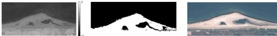
Figure 2.4: NDWI greyscale image (left) and resulting binary image (middle) for a Sentinel 2 image acquired on 12-03-2015 10:33:27 (GMT). The right image shows the same satellite image with the derived SDS plotted in black. (source: adjusted from Hagenaars et al., 2018).
