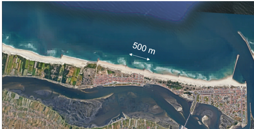
Figure 4.16: Construction of 500-m spaced groynes at a coastal stretch to the south of Aveiro port. (Source: Google Earth).
