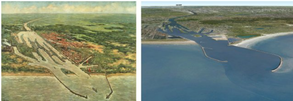
Figure 2.27: Port of IJmuiden in 1880 (left) and the layout of the port in 2005 (right). Accretional patterns at both sides of the port can be observed in the present layout. (source: Luijendijk et al., 2011).
