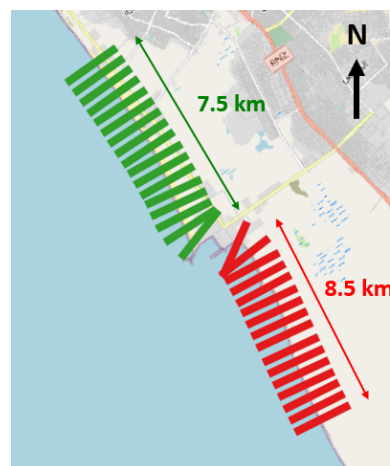
Figure 4.12: Analysed transects at Nouakchott. Accreting (eroding) transects are indicated in green (red). The length up to where the breakwater affects shoreline evolution is also indicated in the figure.
