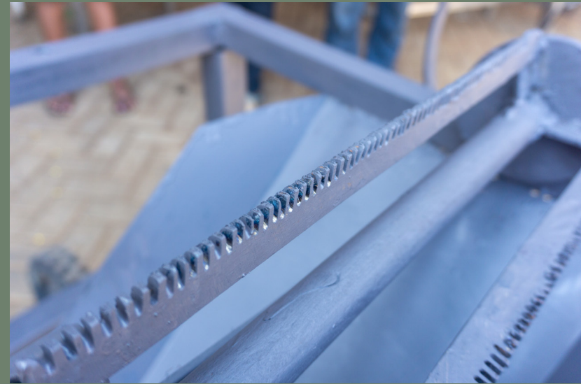
Image 35. Notches in the blades. Photograph by Marte Lanning.
