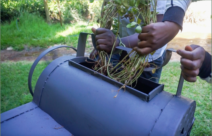
Image 33. Using the safety bar while threshing with the Manual Grounut Harvester. Photograph by Marte Lanning.
