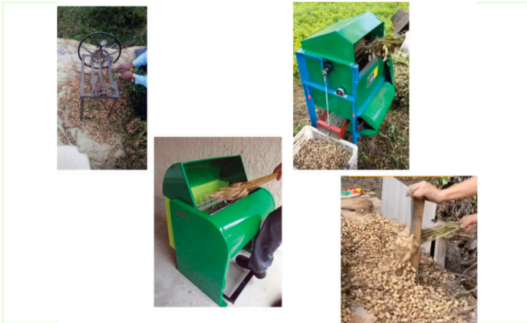
image / figure 1 Current manual threshers worldwide (often expensive, unsafe or still labour intensive).
