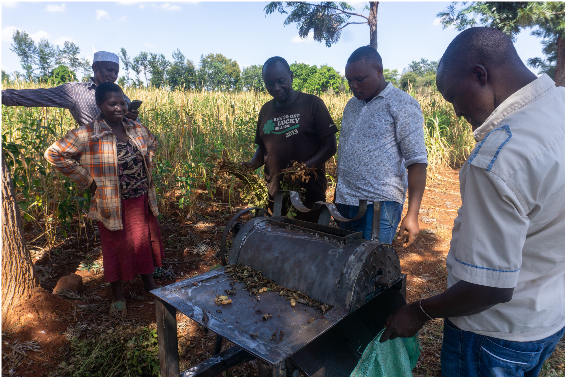
Image 63. Testing the Manual Groundnut Harvester with groundnut farmers Photograph by Marte Lanning.
