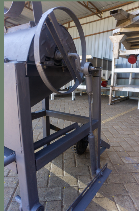
Image 38. Foot pedal connection to pulley and threshing mechanism. Photograph by Marte Lanning.
