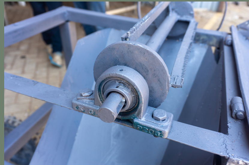
Image 36. Attachment of the shaft and blades to a pulley. Photograph by Marte Lanning.
