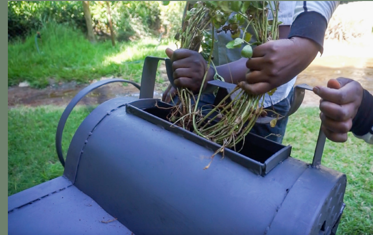
Image 41. Safety bar in use. Photograph by Marte Lanning.
