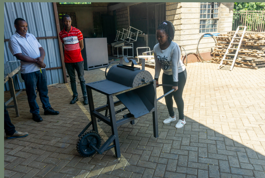
Image 43. Form and transportation of the Manual Groundnut Harvester. Photograph by Marte Lanning.
