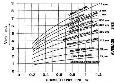
Figure 4.6. Critical velocity according to the MTI model (Eq. 4.19). The nomograph
