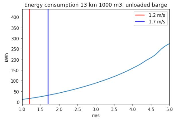
Figure 3.20: Energy consumption unloaded barge 1000 m<sup>3</sup>
