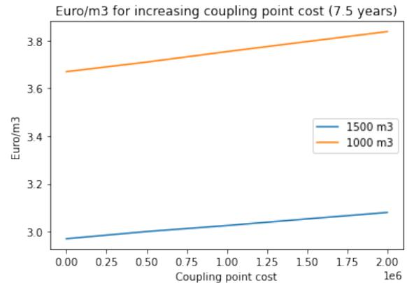
Figure 4.25: Coupling point cost influence on price per cubic meter
