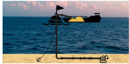
Figure 2.18: Schematization of crawler operation filling a barge
