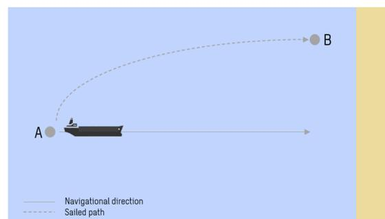
Figure 3.8: Sailing and displacement barge, not symmetrical around tidal velocity
