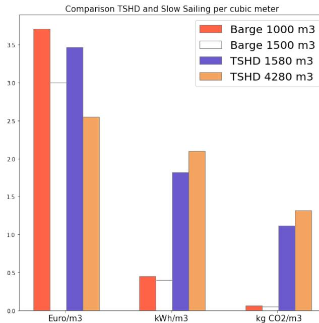
Figure 4.15: Comparison for barges and TSHD's of cost, energy and emissions per cubic meter
