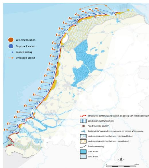
Figure 6.4: Slow Sailing system with moving winning point and disposal location using the residual flow of the tidal velocity
