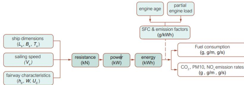
Figure 3.1: Methodology for estimating emissions for IWT vessels mage modified from Segers (2021) by TU Delft Ports and Waterways is licensed under CC BY-NC-SA 4.0).
