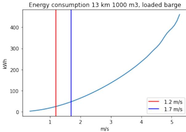
Figure 3.19: Energy consumption loaded barge 1000 m<sup>3</sup>
