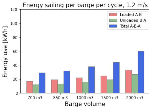
Figure 4.2: Cycle energy consumption barges 1.2 m/s
