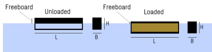
Figure 3.9: Loaded and unloaded situation of barge
