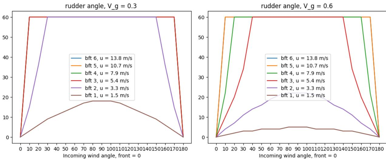
Figure 3.10: Rudder moment compensation angle,  $V = 0.3$  m/s Figure 3.11: Rudder moment compensation angle,  $V = 0.6$  m/s
