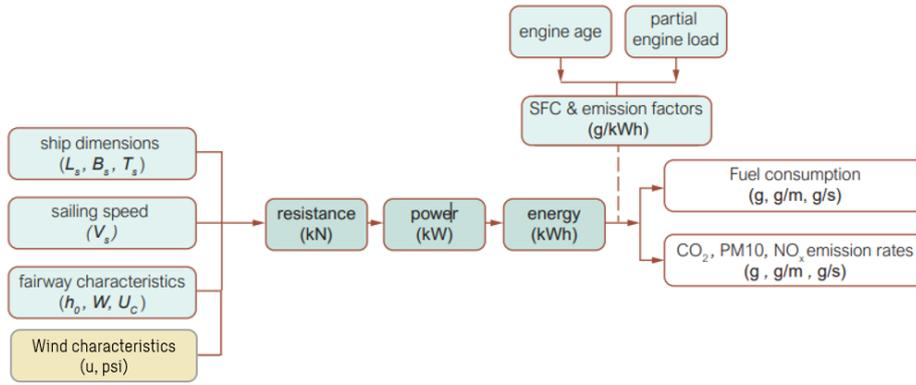
Figure 3.2: Edited calculation scheme OpenTNSim
