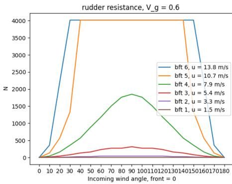
Figure B.9: Rudder resistance,  $V = 0.6$  m/s
