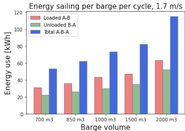
Figure 4.3: Cycle energy consumption barges 1.7 m/s
