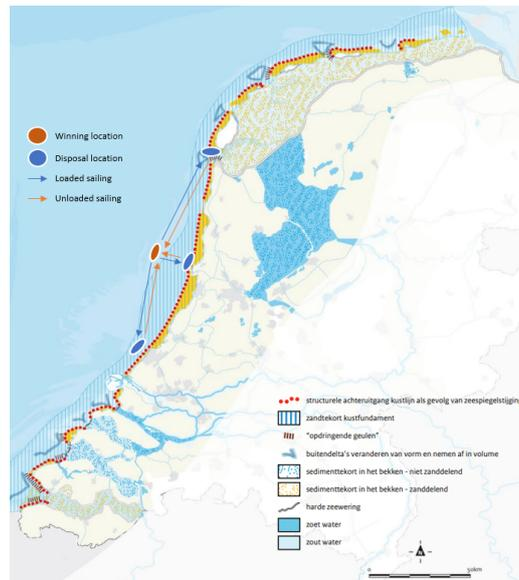
Figure 6.2: Slow Sailing system with multiple disposal locations making use of the tidal motion for alongshore transport
