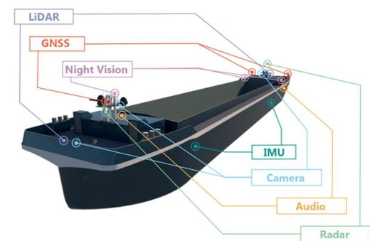
Figure 2.20: Conversion overview barge (Sweco, 2022a)
