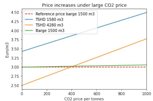
Figure 4.17: Break even price TSHDs and barges under increasing CO<sub>2</sub> price
