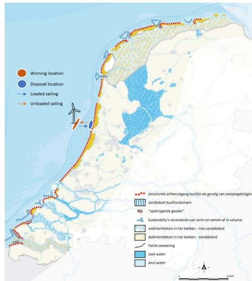
Figure 6.5: Sandwindmill combination with Slow Sailing
