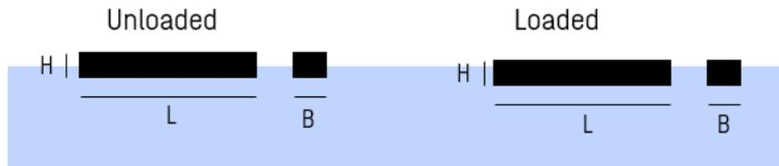
Figure 3.3: Barge schematization overview
