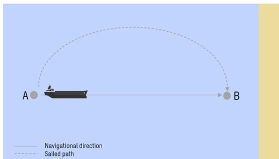
Figure 3.7: Sailing and displacement barge, symmetrical around tidal velocity
