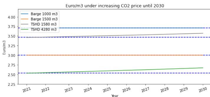
Figure 4.16: Cost increases TSHDs and barges under known CO<sub>2</sub> price increase
