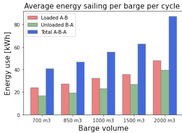
Figure 4.4: Cycle energy consumption barges average speed
