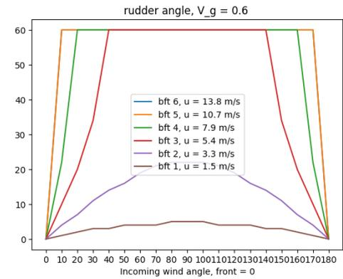
Figure B.16: Rudder angle,  $V = 0.6$  m/s
