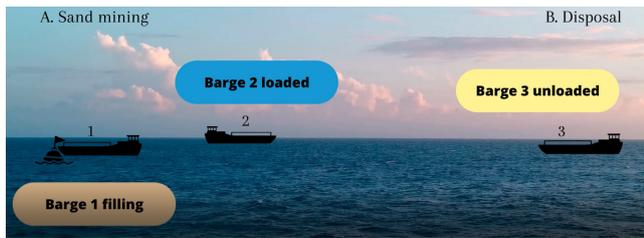
Figure 2.17: Three barges, each in a different phase of the dredging cycle
