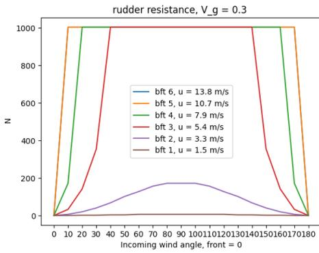
Figure B.7: Rudder resistance,  $V = 0.3$  m/s
