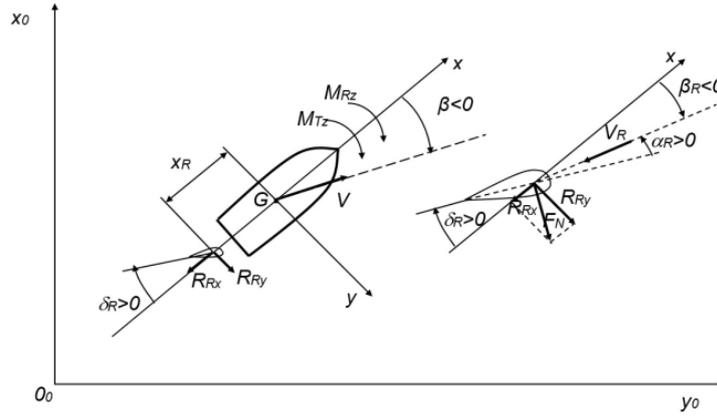
Figure 3.6: Momentum influence on barge and rudder angles
