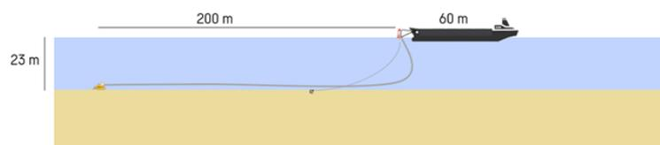
Figure 2.21: Schematic overview anchoring and filling of a barge
