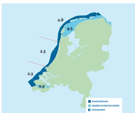
Figure 2.1: Sediment need for Dutch coast subsystems in  $Mm^3$  per year (Rijkswaterstaat, 2021)
