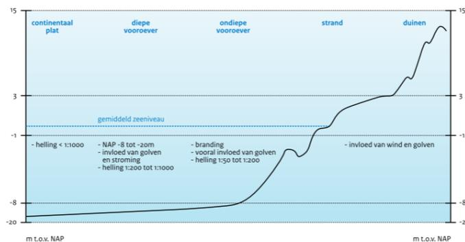
Figure 2.6: Typical dutch coastal depth profile (Rijkswaterstaat, 2020)
