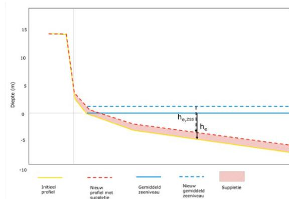
Figure 2.4: Adaptation of profile with sea level rise with suppletion
