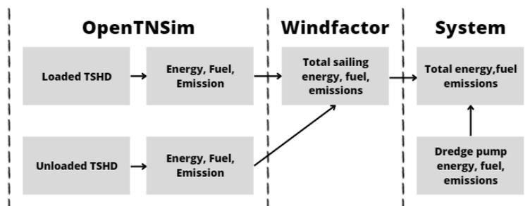
Figure 4.8: Calculation scheme energy use TSHD
