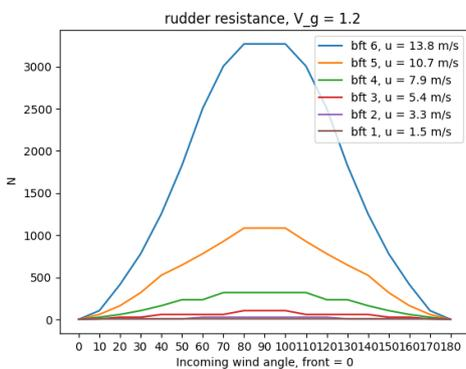
Figure B.11: Rudder resistance,  $V = 1.2$  m/s
