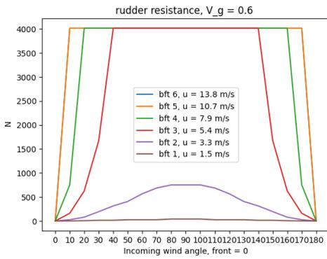
Figure B.15: Rudder resistance,  $V = 0.6$  m/s
