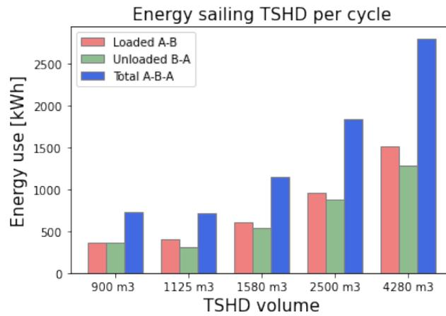
Figure 4.9: Cycle energy consumption TSHD
