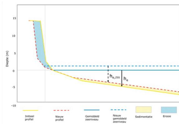
Figure 2.3: Erosion of initial profile with sea level rise without nourishment
