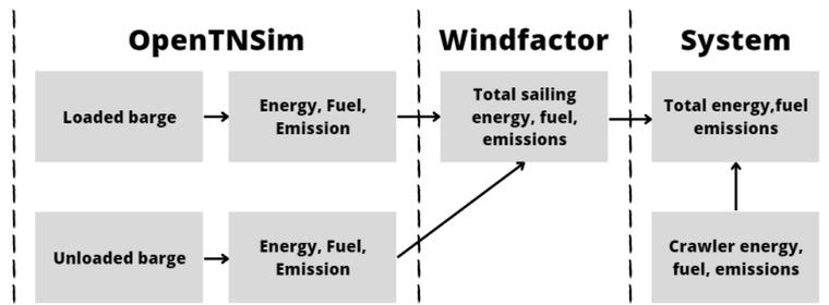
Figure 4.1: Calculation scheme energy use barges
