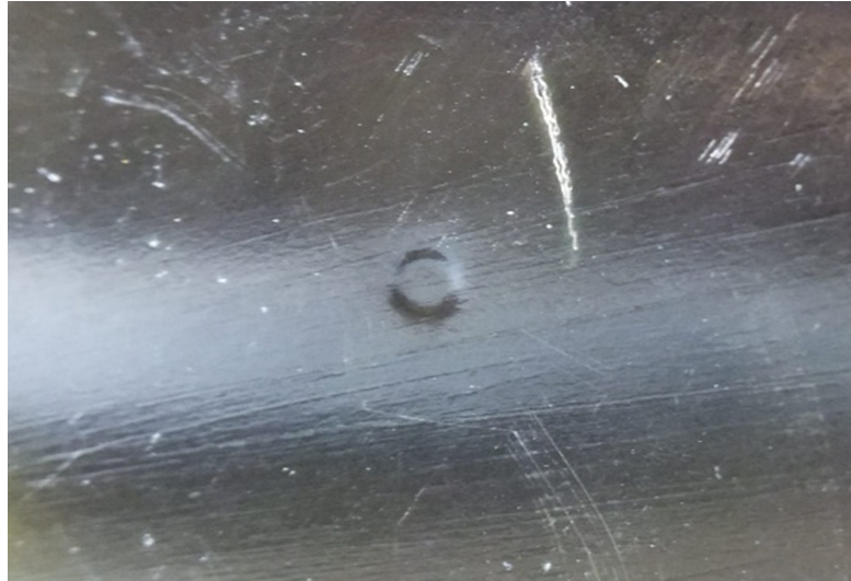
(a) Hardly noticeable BVID from Laminate Outer Surface
