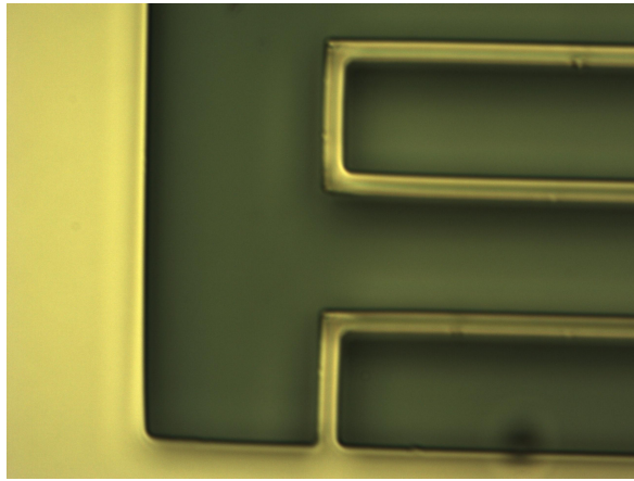
(a) Correct result of a negative photoresist pattern (yellow) over oxide (dark green) of an electrode pair for device W10G02, improved by increased time for x-link bake.
