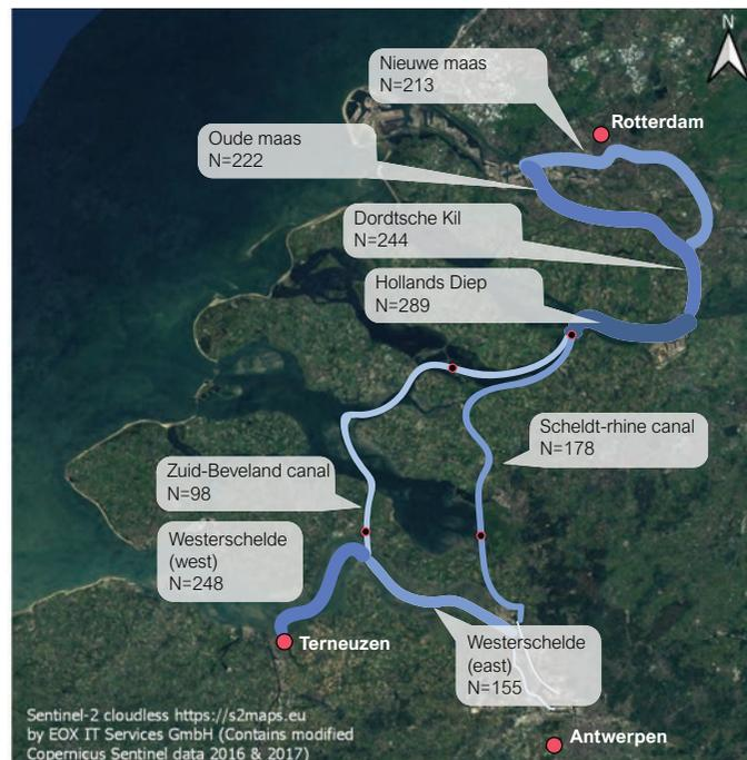
Figure 5.12: Traffic intensity as derived from AIS for the Rotterdam-Antwerp corridor for September 2<sup>nd</sup>, 2019 (image modified from Segers, 2021, by TU Delft – Ports and Waterways is licenced under CC BY-NC-SA 4.0).
