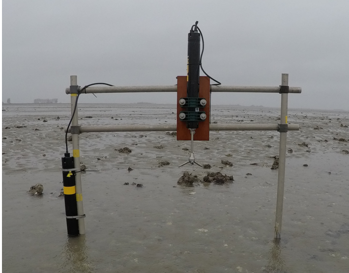
Figure 4.5: ADV frame and additional external battery canister. Taken on 03.02.2021
