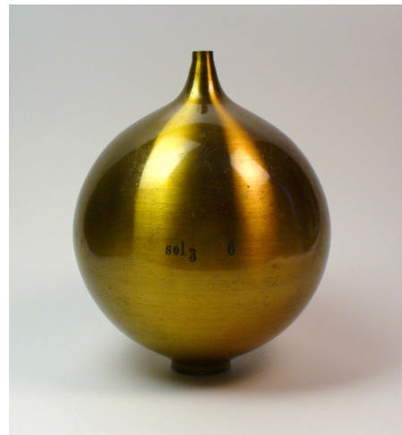
Figure 2.1: A spherical, brass Helmholtz resonator based on the original design. Source: Physics Dept, Case Western Reserve University.
