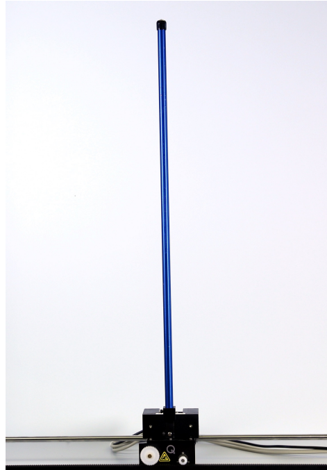
Figure 3-4: Cart-pole testbed used in experiments.
