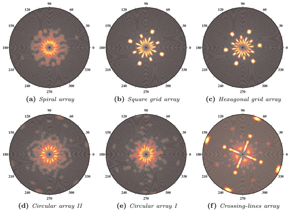
**Figure I.3:** Azimuthal distribution of the receiver pair spacings, represented by their wavenumber equivalents. All figures share the same colour axis. (a) Irregular array based on the Fermat spiral. (b) Square grid array. (c) Hexagonal grid array. (d) Circular array with concentric rings. (e) Circular array with irregular radial growth. (f) Crossing-lines receiver array.
