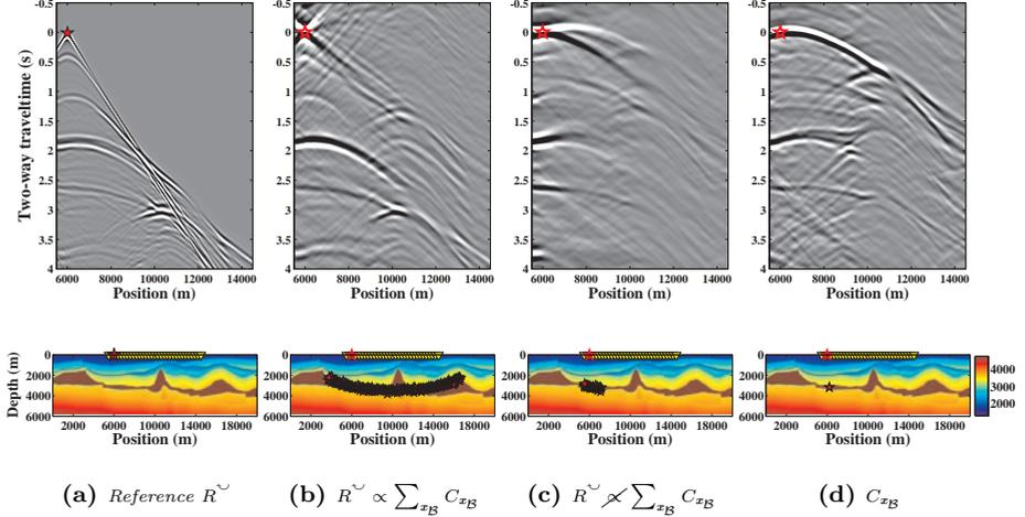
**Figure 4.1:** Three different interferometric results using SI by crosscorrelation. Retrieved shot gathers are shown on top, source distribution inside the acoustic velocity model are displayed below them. (a) Reference reflection response  $R^{\sim}$ . (b) Scenario with equipartitioned illumination from the subsurface. (c) Same result from a limited clustered source distribution. (d) Result obtained from single source in the subsurface.
