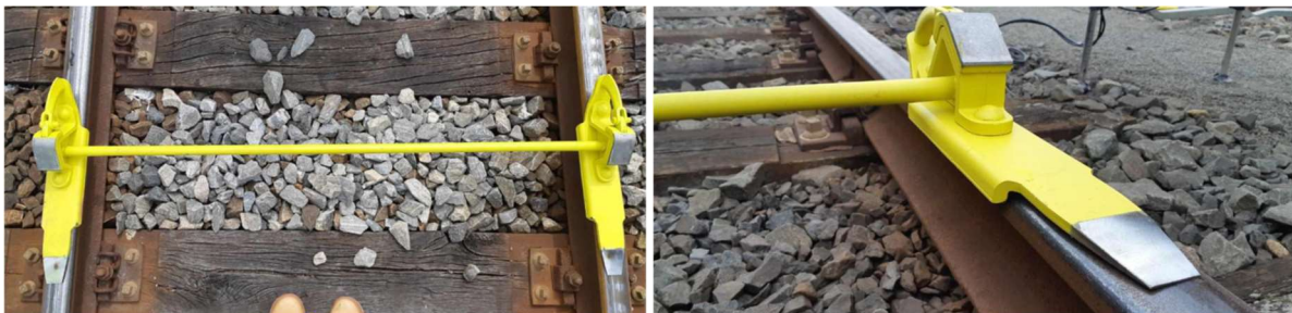
Figure 2.7: The brake shoe at the end of the allocation tracks (Hendriks, 2019).
