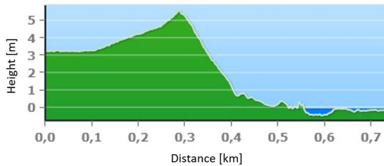
Figure 4.8: Height profile of the hump at Kijfhoek (Home | AHN, n.d.).
