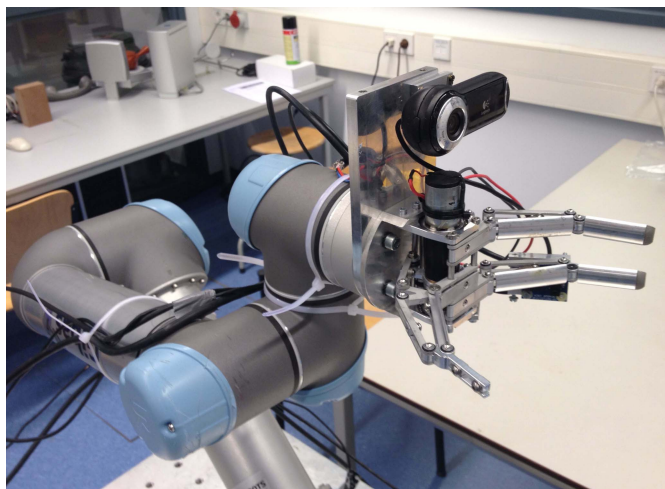
Fig. 11. Eye-in-hand system formed with a UR5 type universal robot arm, a Delft Hand 3 gripper, and a Logitech webcam.
