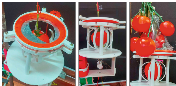
Fig. 7. Shows experiment-2, 3 and 4 i.e. pedicel cutting, grasping and complete operation test respectively.
