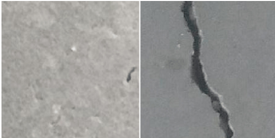
Fig. 1. Two sample images from the dataset: Negative class (no crack) on the left, and Positive class (crack) on the right.
