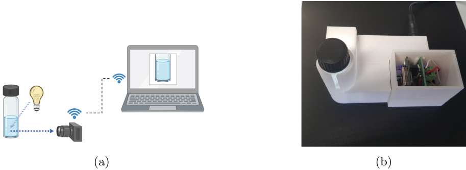
Fig. 2. Experimental setup (a) Schematic representation of the device. (b) Low cost readout system equipped with frugal electronics: in the top-left corner is placed the led. The camera and the embedded system are hosted in the bottom right corner.
