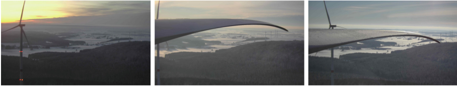
Fig. 1. Exemplary images from the data set: ‘Background’ (left, rotor blades are only in backdrop), ‘rotorblade’ (middle, a rotor blade with no ice) and ‘ice’ (right, a rotor blade with ice).
