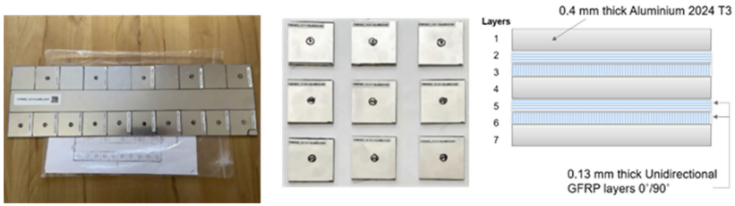
Fig. 3. Fabricated GLARE plate (left) and specimens cut out from the plate to be investigated using X-Ray CT (centre) and a schematic figure of the layup configuration (right).
