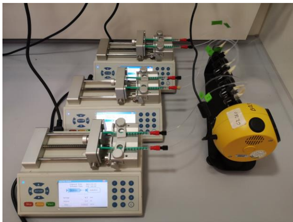
Figure S3.1. Reaction set-up for the enzymatic epoxidation of cis - \beta -methylstyrene. On the left, syringe pumps for continuous t BuOOH supply. Syringes are connected to tubes which lead to the reaction mixture inside GC vials on the right.
