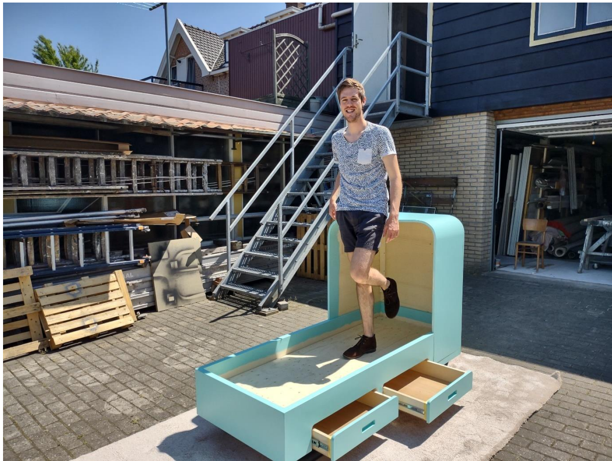
Figure 6.32 - Me standing on one foot on the weakest point of the frame
