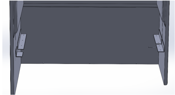
Figure 7.37 - Inserting assembly support brackets
