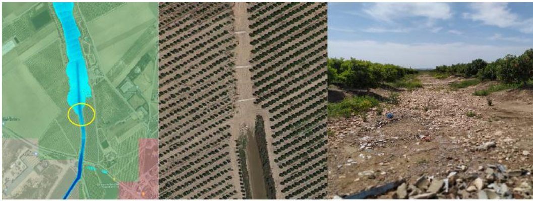
Figure 5.3: Left: Depth map resulting from a scaled flow hydrograph with a maximum of 51 \text{ m}^3/\text{s} . No overflow occurs, which means it determines the maximum capacity of the dry river, if no additional measures are taken to increase the capacity. The flow direction is from the top to bottom of the figure. Middle: satellite image of the terrain, zoomed. The terrain shows that there is an abrupt transition between the farmland and the start of a channel. Right: photo of the river bed taken at upper point of the middle figure, pointed southward.
