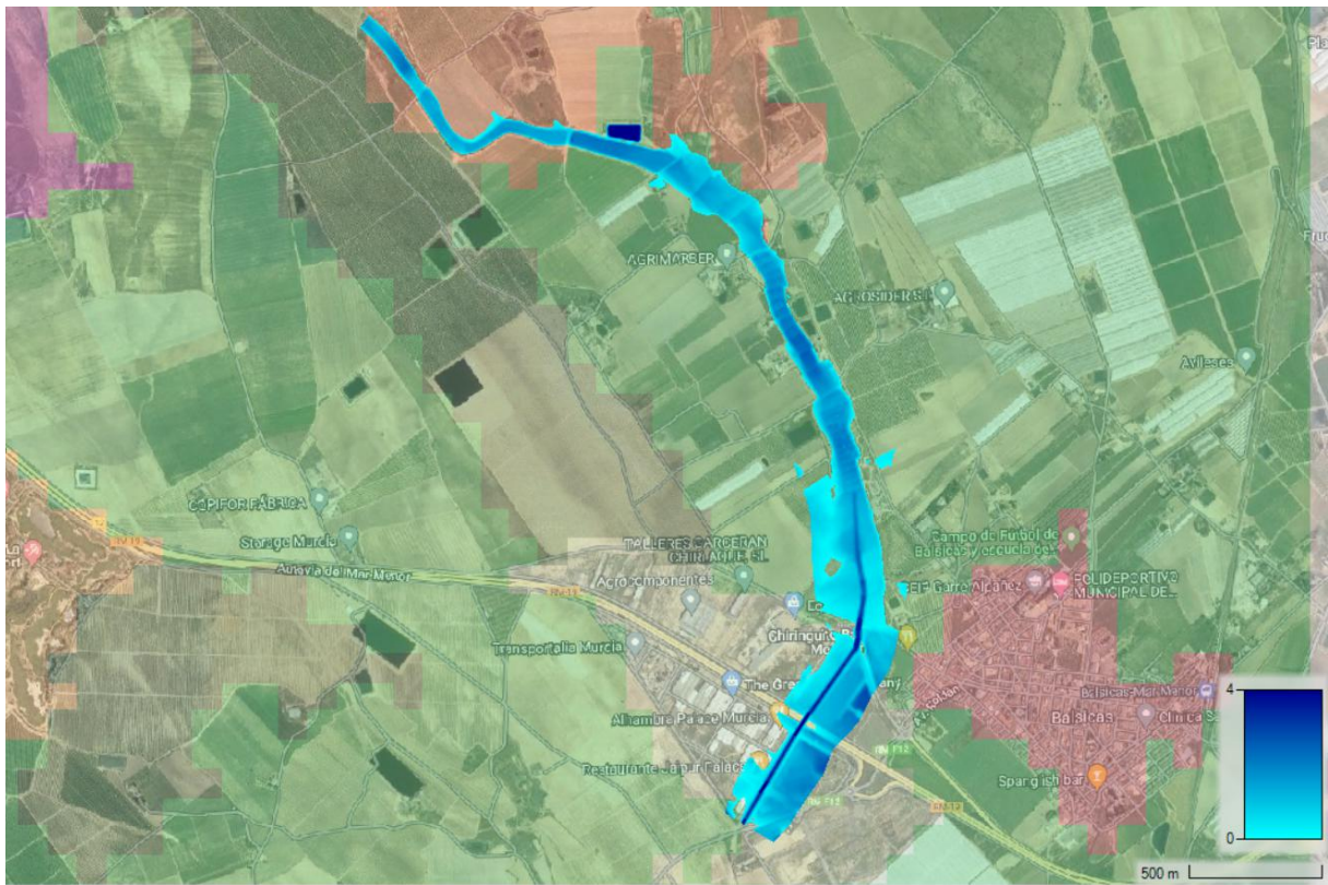
Figure B.1: Depth map resulting from a scaled flow hydrograph with a maximum of 70 \text{ m}^3/\text{s} . This is a complete overview of the dry river reach.
