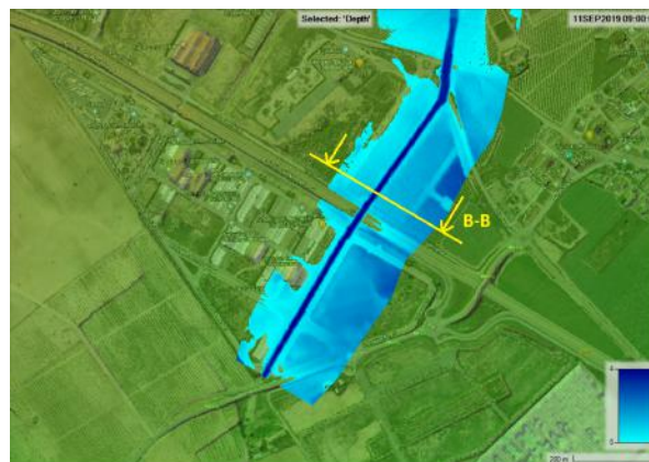
(b) Flow depth map near downstream end of river reach.
