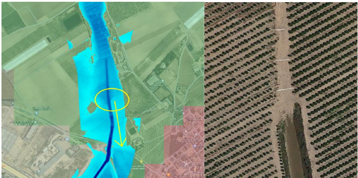
Figure B.2: Depth map resulting from a scaled flow hydrograph with a maximum of 55 \text{ m}^3/\text{s} . This is an overview zoomed on the downstream end of the dry river reach.
