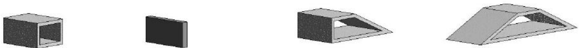
Figure 6.14: 3D view of the considered types of chute spillways. From left to right: Rectangular, Sharp-crested, Right-angled trapezoidal and trapezoidal spillway
