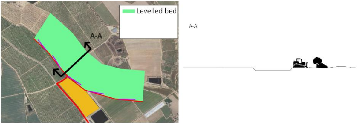
Figure J.3: The next step is cutting trees, removing bushes and leveling the bottom to create a nice working area to build the structure in the existing riverbed. Also the existing road in the most downstream reservoir is removed.
