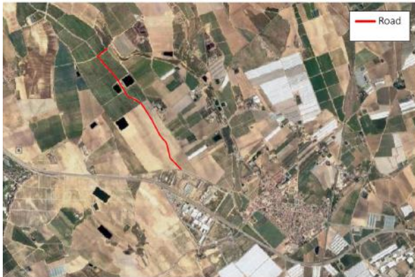
Figure J.1: The red line indicates the route from the main road towards the project location in the north. The almost straight part is an already existing paved road. The last corner is a dirt road of approximately 150 m. The first step is to make the road accessible for all equipment and create a new road towards the ramps to enter the ZAC reservoirs as shown in step 2.
