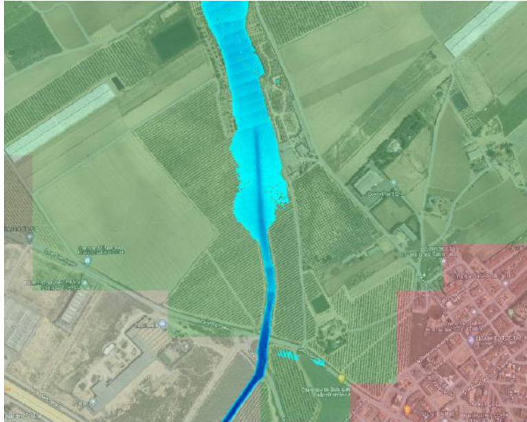
Figure B.3: Depth map resulting from a scaled flow hydrograph with a maximum of 41 \text{ m}^3/\text{s} . No overflow occurs, which means it determines the maximum capacity of the dry river.
