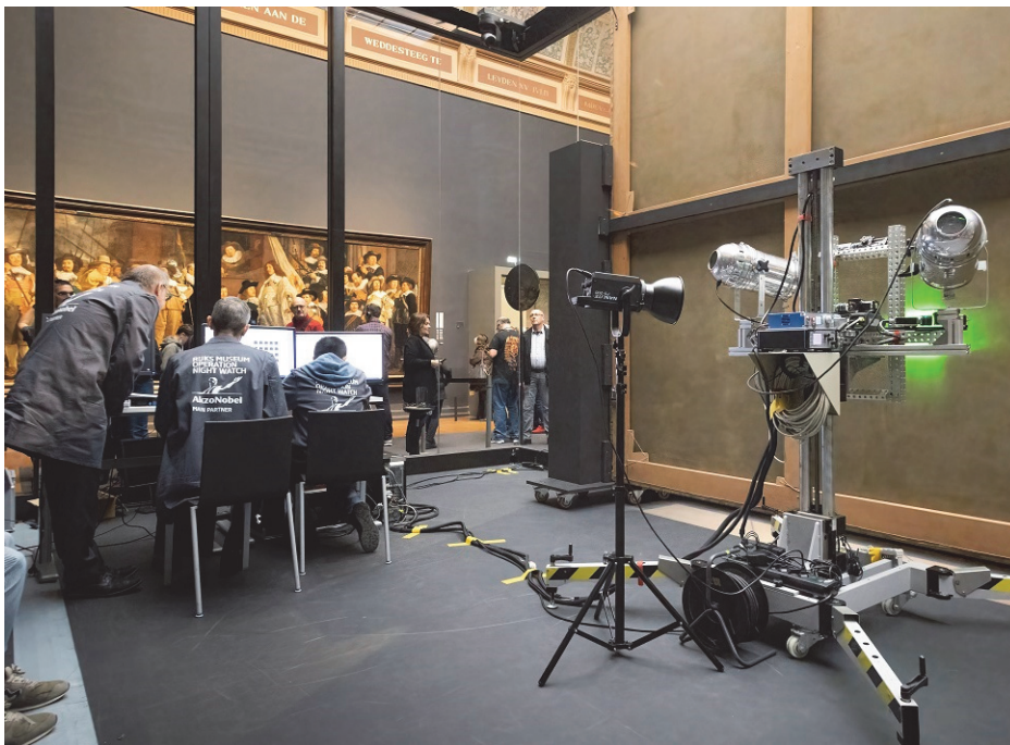
Figure 2. 3D shape shearography instrument positioned behind The Night Watch in the galleries of the Rijksmuseum
