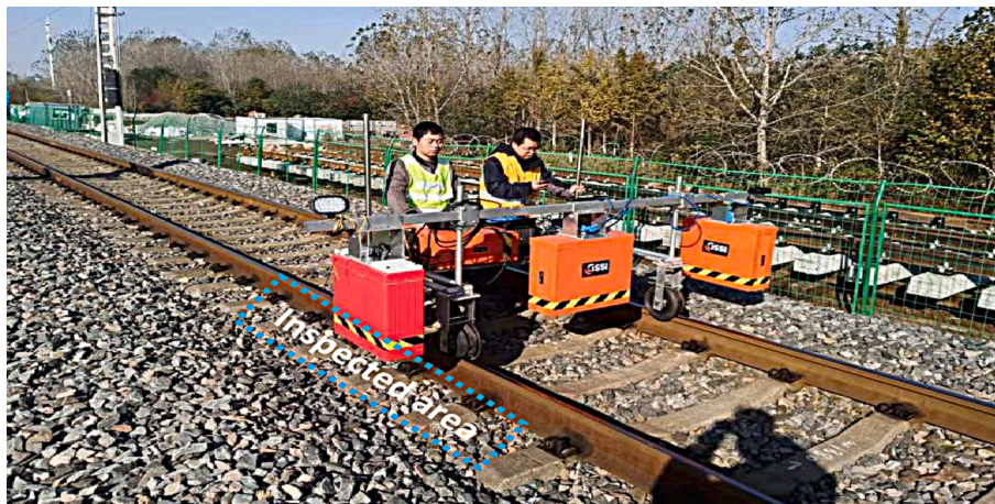
Fig. 1. GPR equipment on ballasted track using 2 GHz antennas.
