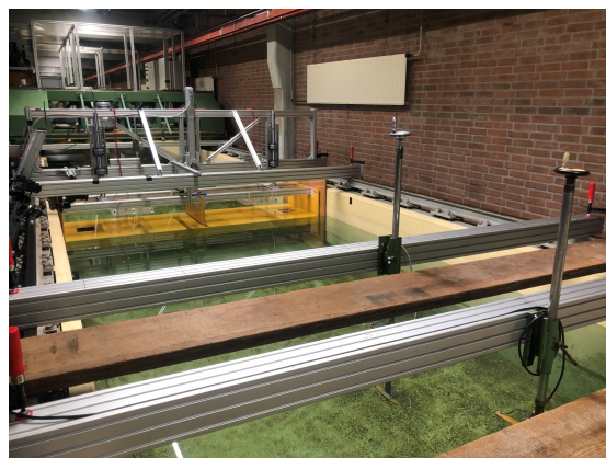
Figure B.5: Overview of setup during wave load tests including two external surface elevation sensors, shot from wave maker side
