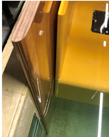
Figure B.9: Gap between the model and the side, approximately equal to 6 mm at each side
