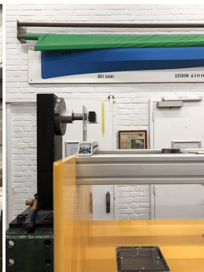
Figure C.2: Close up of the hinge at which the laser for measurements was attached
