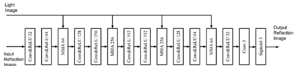
**Figure 2.** Reflectance restoration net.
