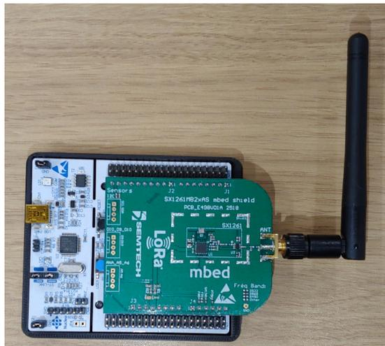
Figure 5.1: **STM32 Nucleo64 F446RE end device with 3D-printed protective case, SX1261MD2BAS LoRa shield, and 868 MHz antenna.**
