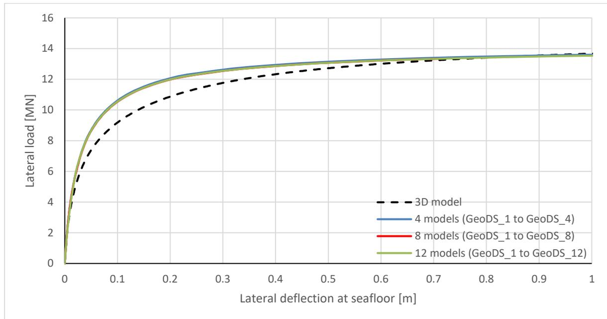
**Figure 4.** Comparison of resulting load-deflection curves for 1D models calibrated with different number of calibration models (see Table 3). The black dashed line represents the equivalent PLAXIS 3D model.
