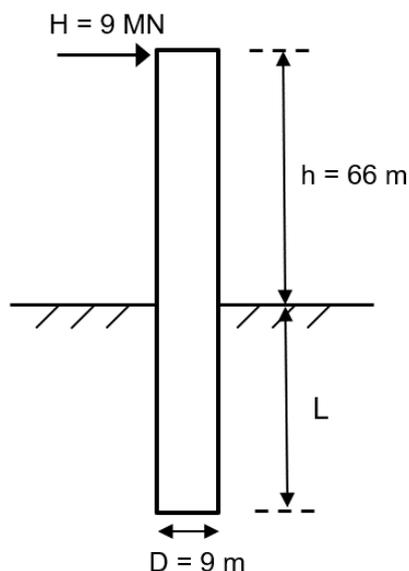
**Figure 2.** Schematic representation of the monopile design.
