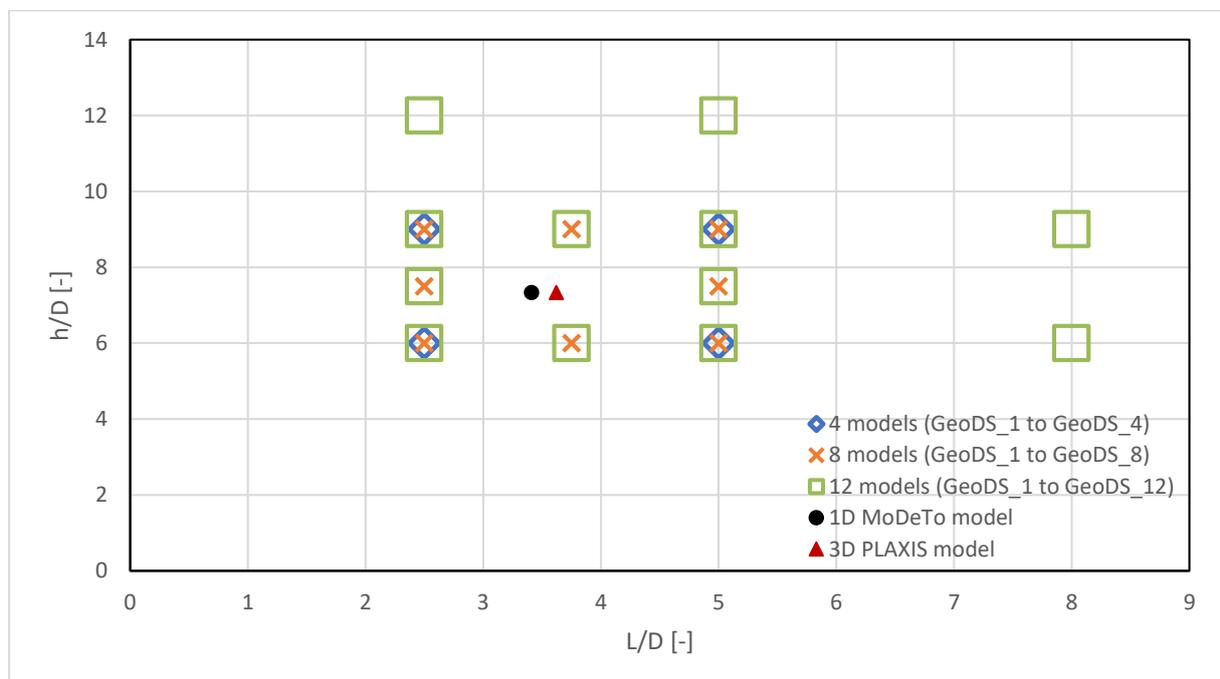
**Figure 3.** Calibration parameter space including the 3D calibration models, the final (optimised) 1D model and the final PLAXIS 3D model ( $h/D$ : load eccentricity ratio,  $L/D$ : aspect ratio,  $h$ : height above seafloor,  $L$ : monopile length below seafloor,  $D$ : monopile outer diameter).
