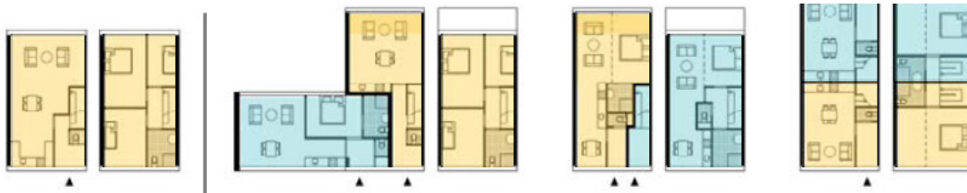
Figure 30 Splitting family row houses (Reimar, et al., 2020)
