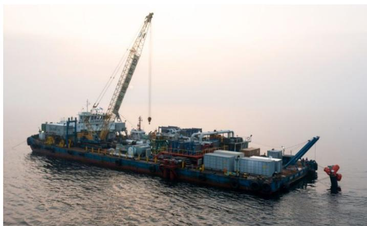
**Figure 2.6:** KRISO's 1-MW K-OTEC 1000 barge [8].
