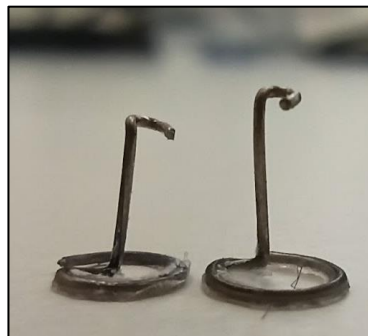
Figure 22. Version 1 and 3 of 3.5 mm model. Left: version 1 ( L_s = 4.10 mm), Right: version 2 ( L_s = 4.65 mm) .
