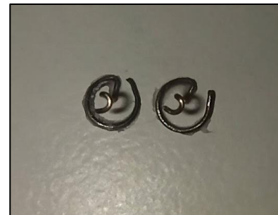
Figure 23. Version 2 and 4 of 3.5 mm. Left: version 2 ( D_h = 3.10 mm), Right: version 4 ( D_h = 3.40 mm).
