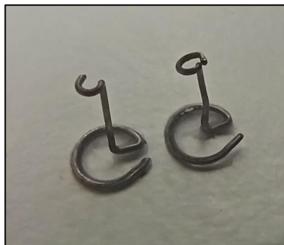
Figure 21. Version 4 and 2 of 5.0 mm model. Left : version 4 ( W_f = 1.00 mm) , Right : version 4 ( W_f = 1.35 mm).
