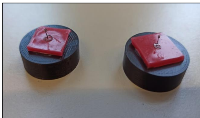
Figure 19. Prepared membrane holders. Left: prepared wire TORP, Right: prepared commercial TORP
