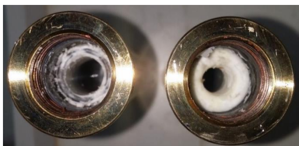
Figure 4-12. 32-day sample tubes, of Surfactant B and Surfactant B+OS, inside metal containers showing a white deposit
