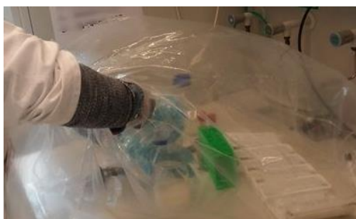
Figure 3-4. Glove bag with Nitrogen or Helium atmosphere and vacuum pump
