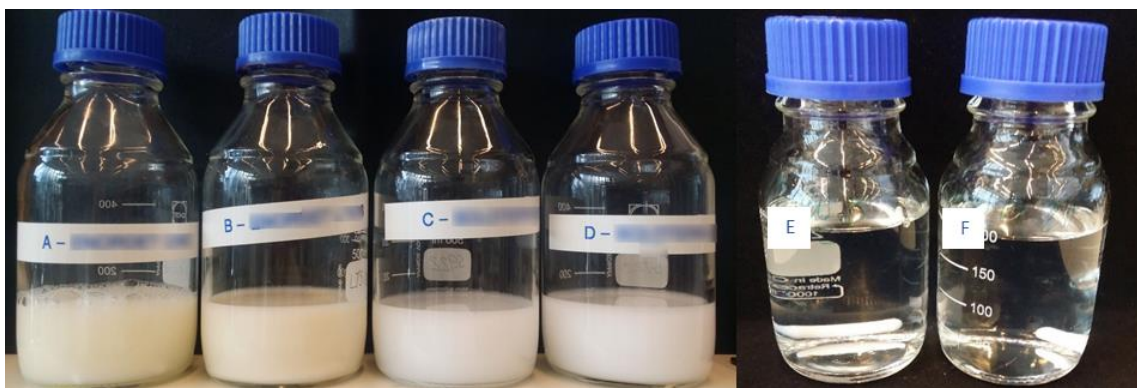
Figure 3-1. Surfactant A, B, C, D E and F diluted at a concentration of 2% wt. of active matter
