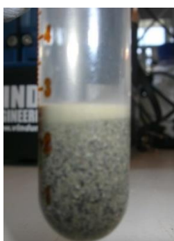
Figure 3-14. Crushed reservoir rock and surfactant solution after being centrifuged
