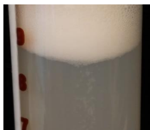
Figure 3-5. Close-up view of foaming (caused by dissolved oxygen) in a 10 ml glass tube after depressurization to atmospheric pressure
