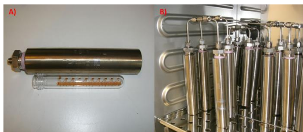
Figure 3-2. (A) Steel holder and 10 ml glass tube (B) Steel holders connected to central gas lines inside oven
