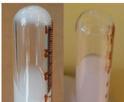
Figure 4-3. Surfactant Bin demineralized before and after heated at 90°C for 24 hours
