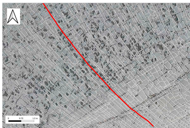
Fig. 12. Continuous and sinuous fracture from Area 4 automatically joined from graph segments with a strike threshold of 20°. Note that the strike of the start and end segment of the fracture vary by more than 50°.
