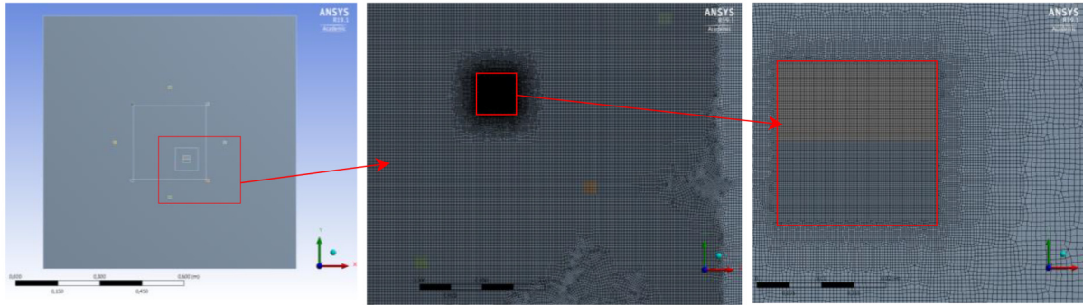
Figure 2. The finite element model of the plate with embedded PZTs and the simulation crack.
