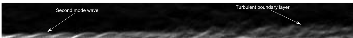
Figure 1.4: Second mode wave visualized on a cone, adapted from Casper et al. [6].
