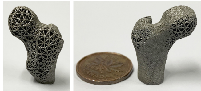
Fig. 15. A bone model with lattice structure generated by our approach as shown in Fig.12 – the metal model is fabricated by a SLM 3D printer).
