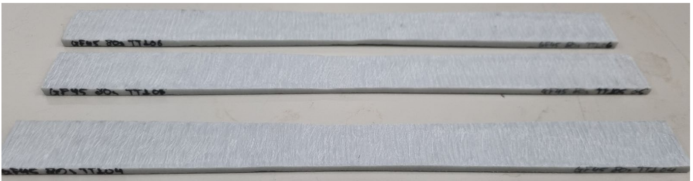
Figure 6-4 Polished coupons of the GF45_80s test series specification
