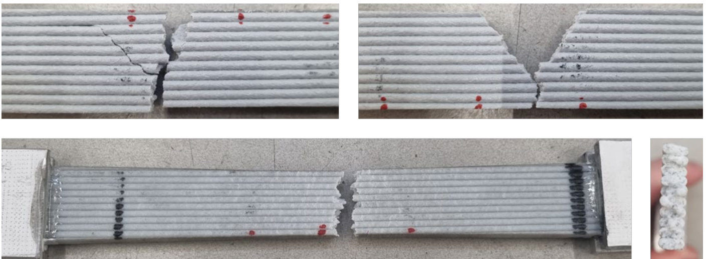
Figure 7-2 Failure mechanisms of coupons tested in tension in longitudinal direction. The two pictures on top are two GF30_80s coupons and the lower the picture are a GF45_80s coupon
