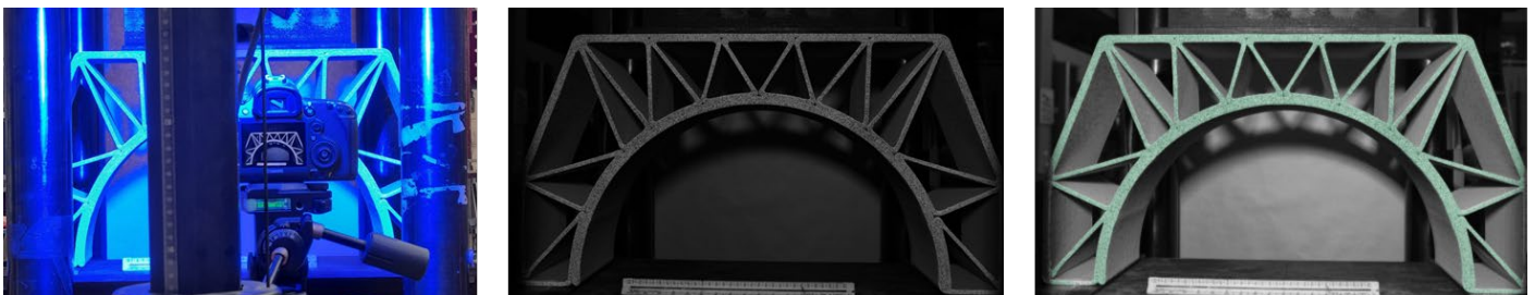
Figure 9-17 Picture from the DIC measurement converted to a surface component plane in the software
