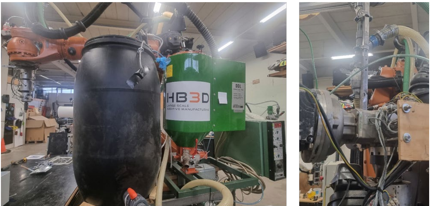
Figure 4-7 Reservoirs in which the granulated material is dried (green) and stored (black) before it goes to the small reservoir (pointed with the red arrow)
