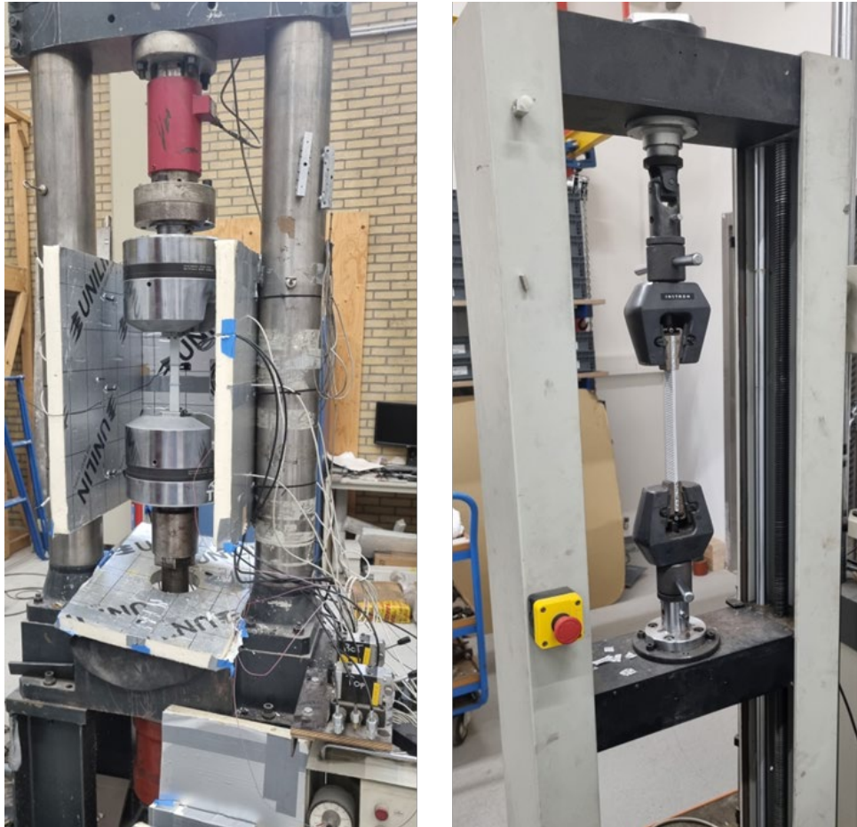
Figure 6-7 Machines used for the first stage of coupon testing. The Dowtey-Rotel machine (left) for the longitudinal tensile tests and the Instron1122 machine (right) for the transverse tensile test
