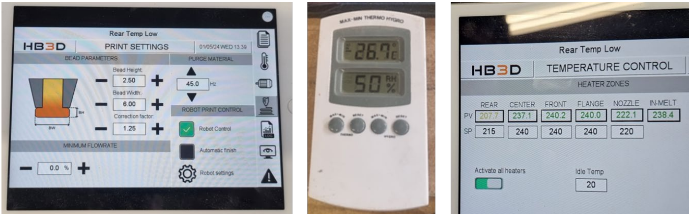
Figure 9-10 Print settings of the bead dimensions (left), the ambient conditions during printing of the two bridge deck components (middle) and the temperatures in the extrusion arm of the printer (right)
