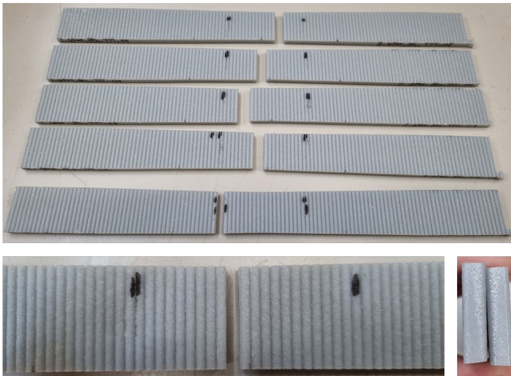
Figure 7-15 Failure mechanisms of the transverse tensile test coupon in the second stage of coupon testing
