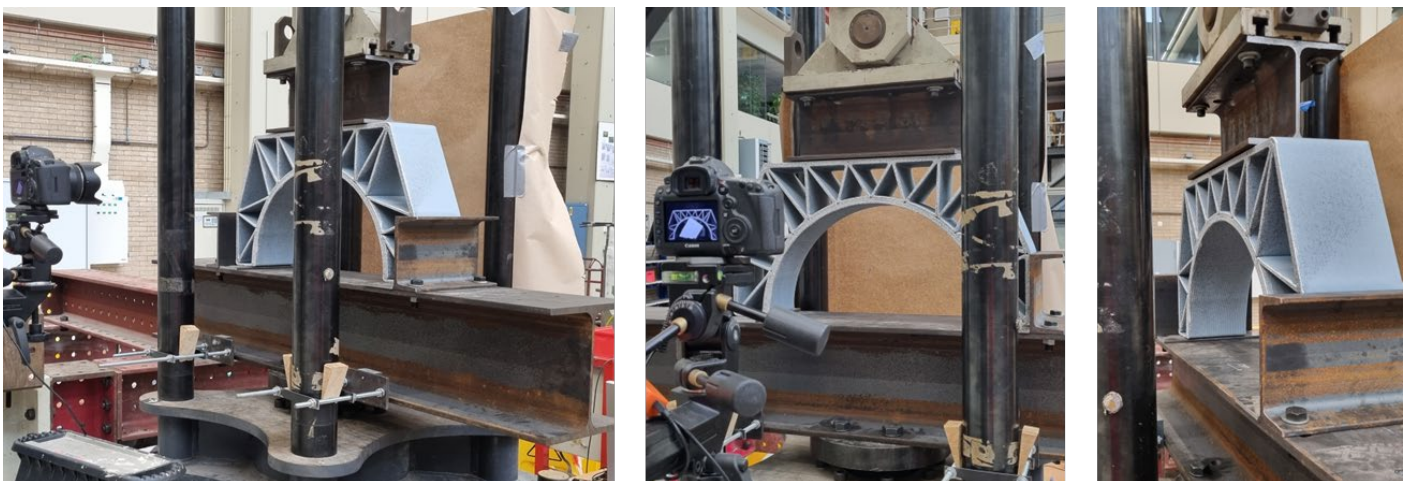
Figure 9-15 Arch component in the test set-up for the simulation of a wheel load with camera and the painted side for DIC measurements
