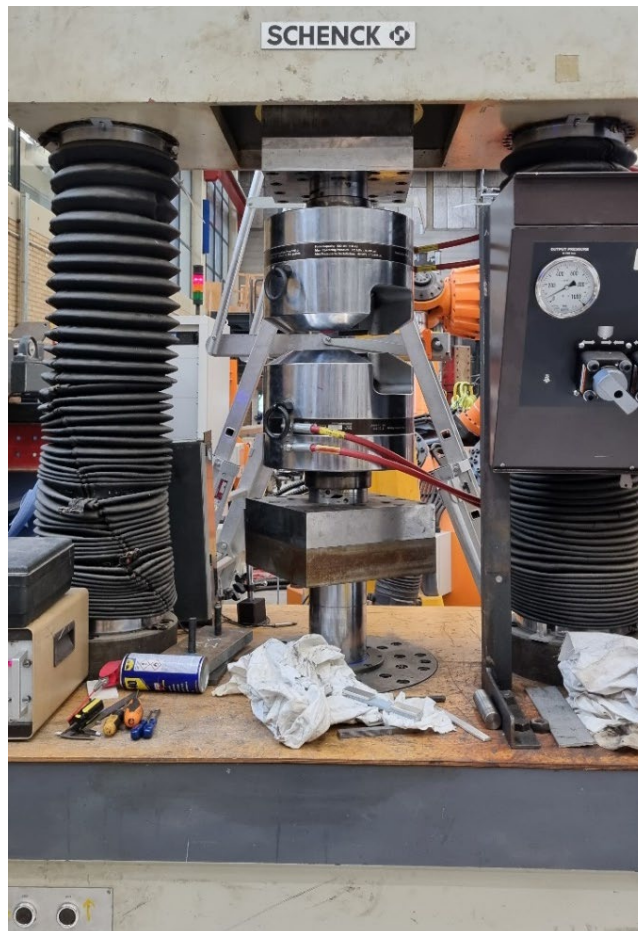
Figure 6-11 Schenk_S_600kn machine used for the compression tests
