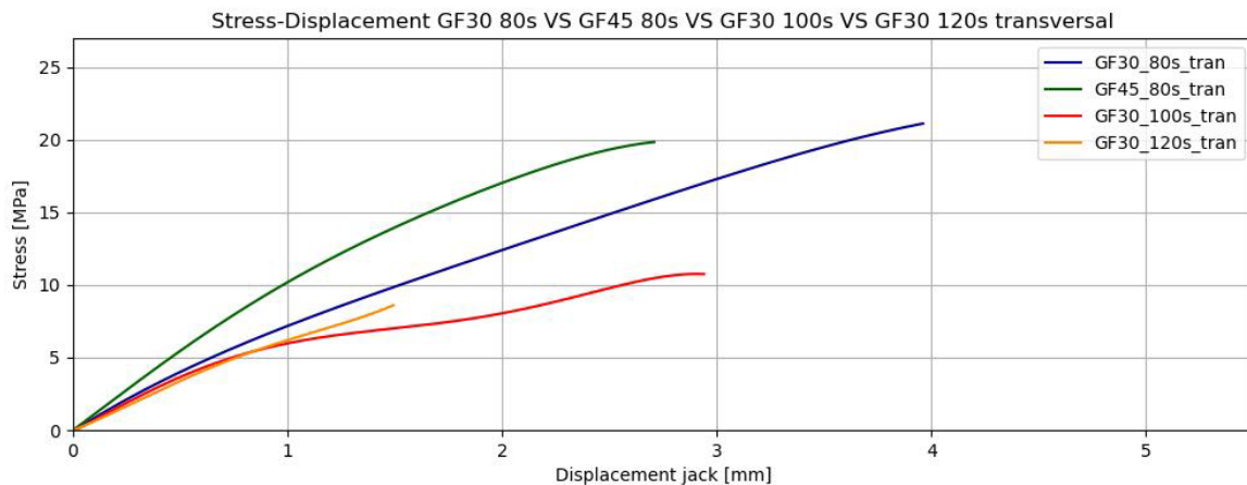
Figure 7-5 Stress-displacement diagram of the tensile test results of GF30_80s, GF45_80s, GF30_100s, and GF30_120s in transverse direction
