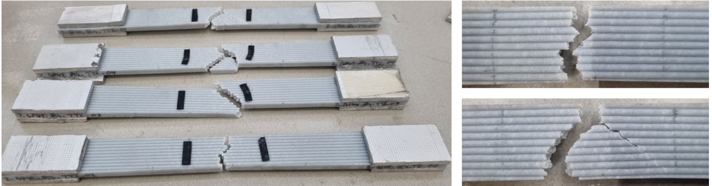
Figure 7-12 Failure mechanism of some of the longitudinal tensile test coupons in the second stage of coupon testing
