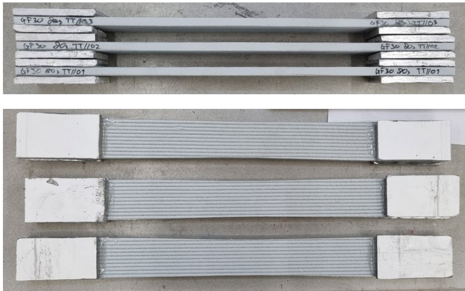
Figure 6-5 Longitudinal tensile coupons GF30_80s with aluminium tabs glued on the clamping surface
