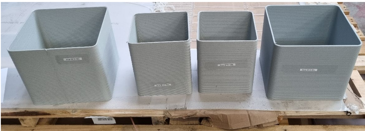
Figure 6-1 The four 3D printed boxes for the first stage of coupon testing ready to cut the specimens from
