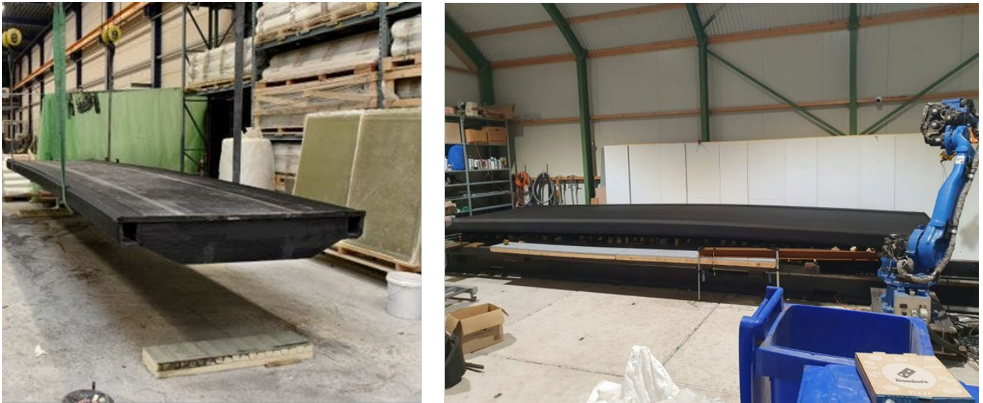
Figure 2-4 3D printed bridge by 10XL in the factory [10]
