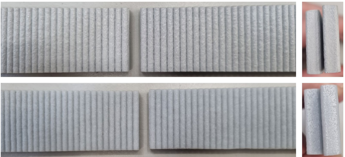
Figure 7-4 Failure mechanisms of coupons tested in tension in transverse direction. Both GF30_80s (above) and GF45_80s (below) failed in between the print layers
