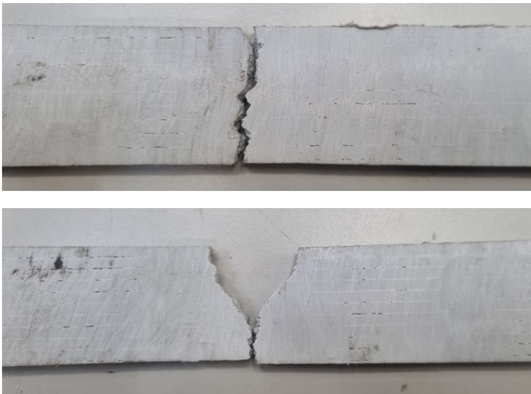
Figure 7-9 Failure mechanisms of two GF30_80s coupons tested in longitudinal tension after polishing
